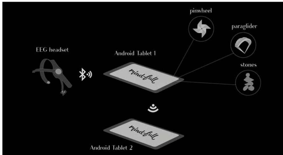
Fig. 1. System Configuration.
