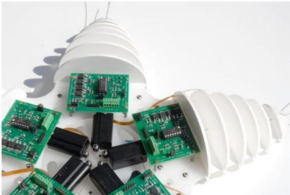
**Figure 3 Actuators and driver boards**
